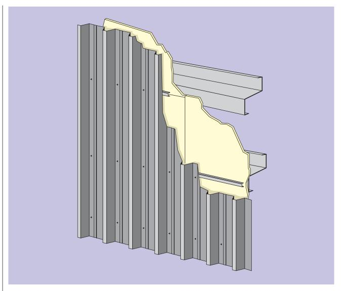
The **Stramit Uniquard™ fire-resisting wall system** combines a single Promina®60 board with profiled steel wall cladding. The strength, simplicity and thermal insulation properties of the system make it an ideal boundary wall solution for industrial and commercial buildings.
