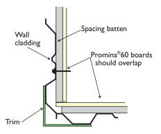
See product technical manuals for Stramit® Corrugated, Monoclad® or Longspan® steel cladding, or the Stramit® Roof & Wall Flashing Design Guide for further flashing, trim and moulding options.
