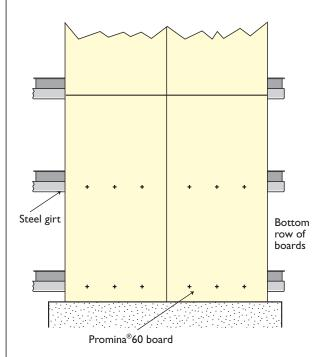
N.B for the two outer screws leave a minimum of 100mm gap from board edge.
