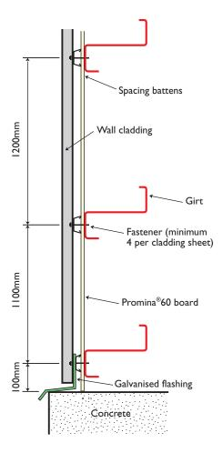
The gap between the concrete floor and the bottom row of boards should be no more than 5mm.
