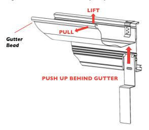
4. While holding down the Stramit® Gutter Spacer flat against the Stramit® Fascia Board, pull down on the Stramit® Inserting Tool to position the hooks of the Stramit® Gutter Spacer over the back of the gutter. Tilt the hand held part of the Stramit® Inserting Tool away from the Stramit® Fascia Board to disengage the lower hook and pull down to remove the tool.
