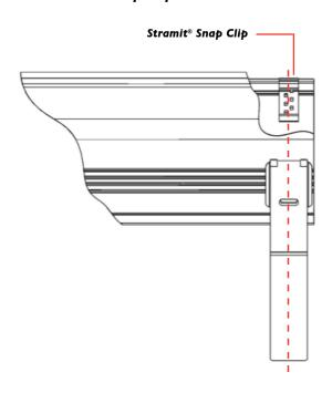
3. While gently lifting up and pulling away on the bead of the gutter to generate a gap between the gutter and fascia board, push the **Stramit® Gutter Spacer** up behind the gutter while making sure the spacer is aligned with the **Stramit® Snap Clip**.
