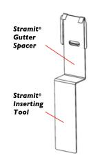
2. Align the Stramit® Gutter Spacer with the Stramit® Snap Clip.
