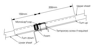
3 Screw down the sheeting as per normal practice at all supports except at the joint. Turn up the high ends of the lower sheet in every pan using the MonoLap® roof lap joint turn-up/down tool.
