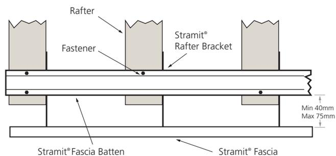
Alternative fastener location at internal supports
